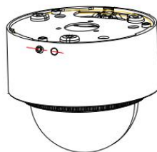
Figure 2-13 Fit Camera to Bracket
